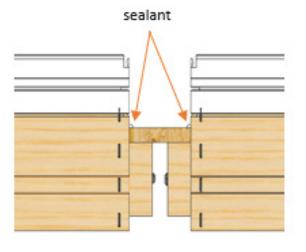
Place a bead of silicone sealant along both edges of plywood where it meets the window.
