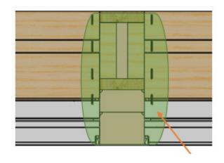
Fill all gaps in mull system with sealant on both ends of the mull.
