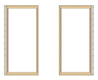
Lay the units down on a drop cloth or cardboard in the order they are to be mulled with exterior side down. Pull off the head, sill, and jamb nail fins from each unit where the mull will connect them.
