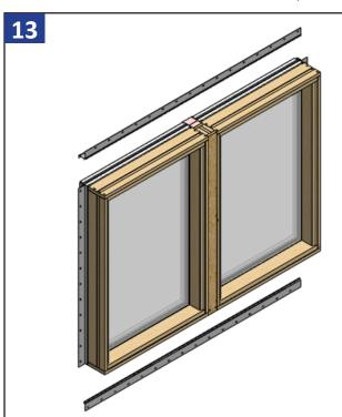
Install new full length head and sill nail fins.
