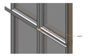
If there are horizontal and vertical mulls on the application, make sure that the joint where the two mulls meet is back bedded with a generous amount of sealant before sliding mull cap into place.
