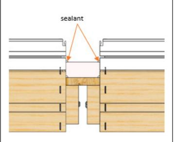
Install foam installation board over plywood and place a bead of silicon along the edges.
