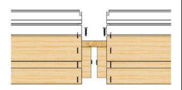
Move the window units together with a 2'' (for 2'' mull) or 4'' (for 4'' mull) gap to allow for plywood caps. Exterior side up.
