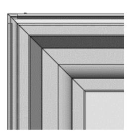
Cut a notch in the exterior clad accessory channels in the head and sill to allow for mull key to set flush. If not already done from the factory.
