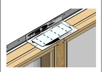
Install mending plate centered over mull gap and staple or screw into place. (Do not use fasteners longer than 34")
